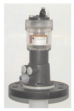
KCI reservoir mounted on top of the assembly CPA 140
