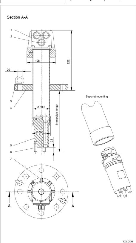
Dimensions of the stainless steel assembly DipFit P CPA 140
